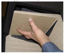
The smoke barrier rests on 2 pins in the back and 2 spikes in the fitting in the front.
