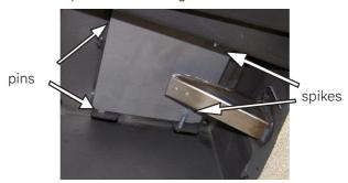
Lift off the smoke barrier, pull forward, lower and remove.
