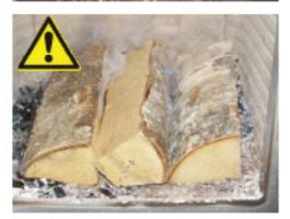
Here firewood has been added to an ember layer which is too small, and the air flow is too small - smoke is developed.
