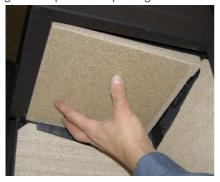
Then, lower the front corner and carefully pull out the plate.
