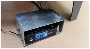
Place the receiver on the two fasteners under the burning chamber when mounting the burner assembly.
