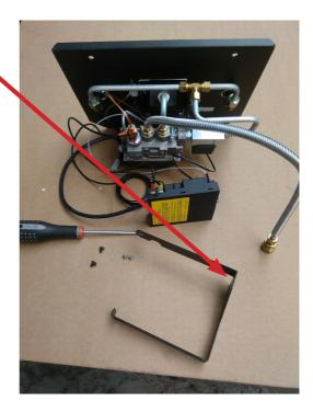
Remove the receiver plate which is hanging under the stove
