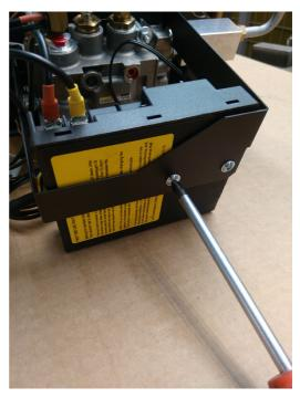
Unscrew the receiver bracket from the burner assembly.
