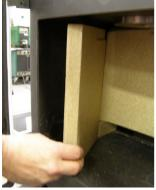
2. The bottom plate is gently lifted out of its position with f. ex. a wide slotted scruedriver.
