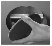
Remove the blanking plate and the packing, and position them in the hovle at the top. Ensure that the packing is positioned correctly. Screw all elements together with the three M6 nuts.
