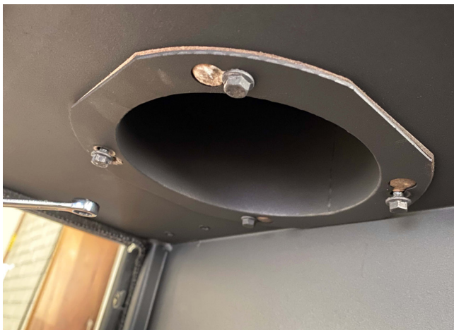
1. Loosen two of the bolts diagonally.
